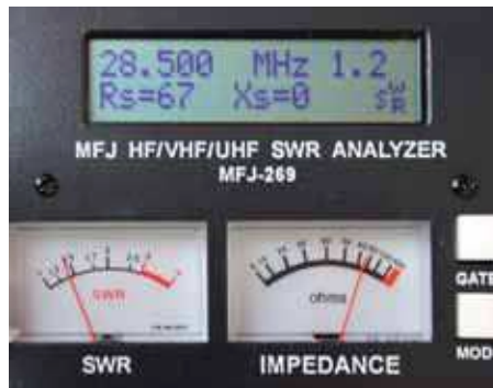
PHOTO 2: At resonance the aerial is quite well-behaved.
